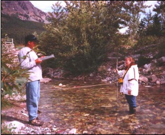
Figure 7. Stephanie Running Wolf of the EPA with a Blackfeet Tribe intern measuring the stream discharge in Rose Creek (GNP1). Middle Fork of the Flathead River on August 21, 2002. Water quality parameter measurements and water samples were also taken on August 21, 2002 from the north exterior spigot of the Fire Cache Building, which is piped approximately 100 feet from a water infiltration gallery from under Bowman Creek. All water samples were taken in accordance with MDA's standard operating procedures. All of the surface water samples were analyzed using a Phenoxy Multi-Residue method, which includes the most commonly used pesticides in GNP of 2,4-D, Clopyralid, Picloram, and Triclopyr. For the complete list of analytes included in the Phenoxy Multi-Residue method see Appendix C.
