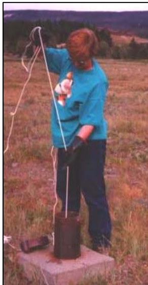
Manager for MDA, bailing St. Mary USGS monitoring well (GNP4).
